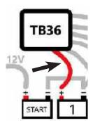
10. The RED cable is connected to the positive (+) terminal of trolling motor battery 1. On 3 battery systems this is also the starter motor positive (+) connection. Extending this wire with 8- or 6-gauge wire can be done, if necessary.
