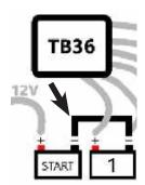
8. On a 4 battery system with isolated starting battery, connect the negative (-) of the starting battery to the negative (-) of trolling motor battery 1.
