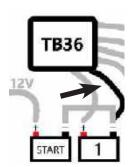
9. Connect the BLACK Trollbridge 36 ground wire to the negative (-) terminal of trolling motor battery 1. This terminal also connects to the negative (-) of the starting battery and the negative (-) side of the trolling motor. Extending this wire with 8- or 6-gauge wire can be done, if necessary.
