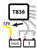
11. The YELLOW cable is the incoming charging line and will be connected to the positive (+) of the starting battery. When extending the wire length use no heavier than 10 gauge up to ten (10) feet and 8 gauge over ten (10) feet. On a 3 battery system connect YELLOW cable to the trolling motor battery 1 positive (+) post with the red wire from the Trollbridge 36.
