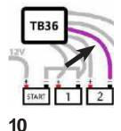
12. Connect the PURPLE cable to trolling motor battery 2 negative (-). Extending this wire with 8- or 6-gauge wire can be done, if necessary.
